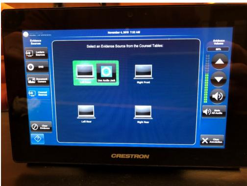
The touch panel works by simply pressing on the desired input. Once pressed, the connected device will automatically publish to the courtroom evidence monitors. The control panel also contains a volume control setting, a mute button, a clear annotation button (if annotations have been made), and a clear evidence button (which will blank the evidence monitors).
