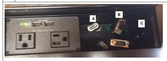
Gently **extend** desired cable from the cable cubby in the cart > Plug **equipment** (e.g., laptop) into the Presentation Cart using the corresponding cables (Explained below):
