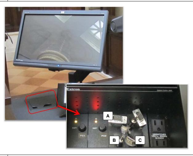
**2** Gently **extend** desired cable from the cubby hole in the cart > Plug **equipment** (e.g., laptop) into the Presentation Cart using the corresponding cables (Explained below):
